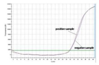
Figure 2: The positive sample as well as the negative sample show a signal in the Control RNA-specific  $VIC^{\oplus}/HEX/JOE^{TM}/TET$  channel. The amplification signal of the Control RNA in the negative sample shows, that the missing signal in the virus-specific FAM channel is not due to RT-PCR inhibition or failure of RNA isolation, but that the sample is a true negative.
